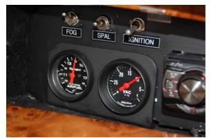
Fig. 11 - AFR and manifold vac. gauges
