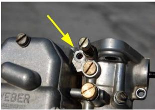
Fig. 4 - Manifold vacuum access point
